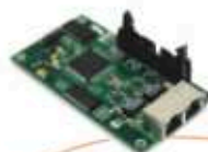
Pluggable Interface Module PIM-2Eth-U* (interface 2xEthernet)
